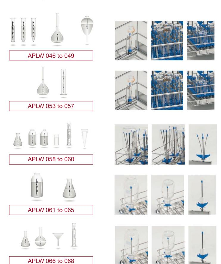
Depending on the form and size of loads, injector nozzles should be chosen to give a gap between the tip of the nozzle and the base of the glass of between 10 and 90 mm. Various nozzles can be supplied with a spring clamp for height adjustment. By adjusting the spring clamp, it is possible to reprocess laboratory glassware in a variety of sizes.
